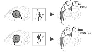
• Check the selector knob for proper function. (When rotated, the cam offers more resistance in the lead climbing position than in the top-rope position).
