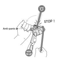
3. Checking the anti-panic on the GRIGRI +. Hang from a low height. Pull the handle QUICKLY while holding the brake-side rope. The rope should be locked.
