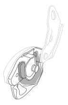
• Verify the absence of foreign objects (sand...) or lubricant on the rope channel.
