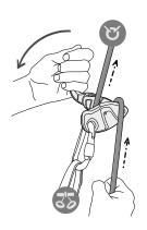
2. Hang from a low height. Pull the handle while holding the brakeside rope. The rope must slide through the device.
