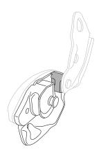
• Check the condition of the friction plate (marks, deformation, fouling, cracks...).
