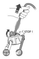
1. Pull on the climber-side rope; the device should lock the rope.
