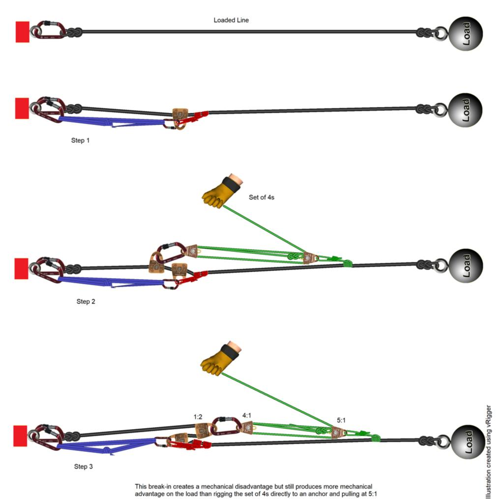
This break-in creates a mechanical disadvantage but still produces more mechanical advantage on the load than rigging the set of 4s directly to an anchor and pulling at 5:1
